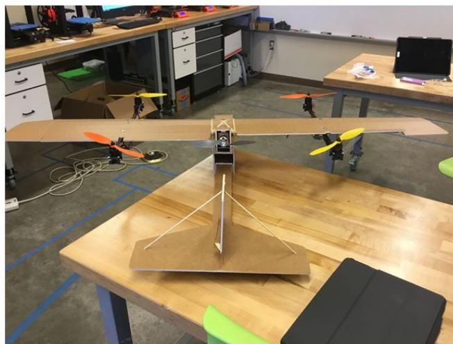
Fig. 2: Our VTOL plane from the back; the pusher motor has the gray propeller and is positioned in a different direction to drive the plane forward during fast forward flight.
