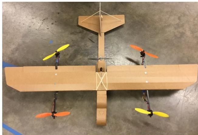
Fig. 1: The top view of our VTOL plane; the four hover motors are those with yellow or orange propellers.
