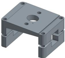
Figure 7: V3 Back Motor Mount
